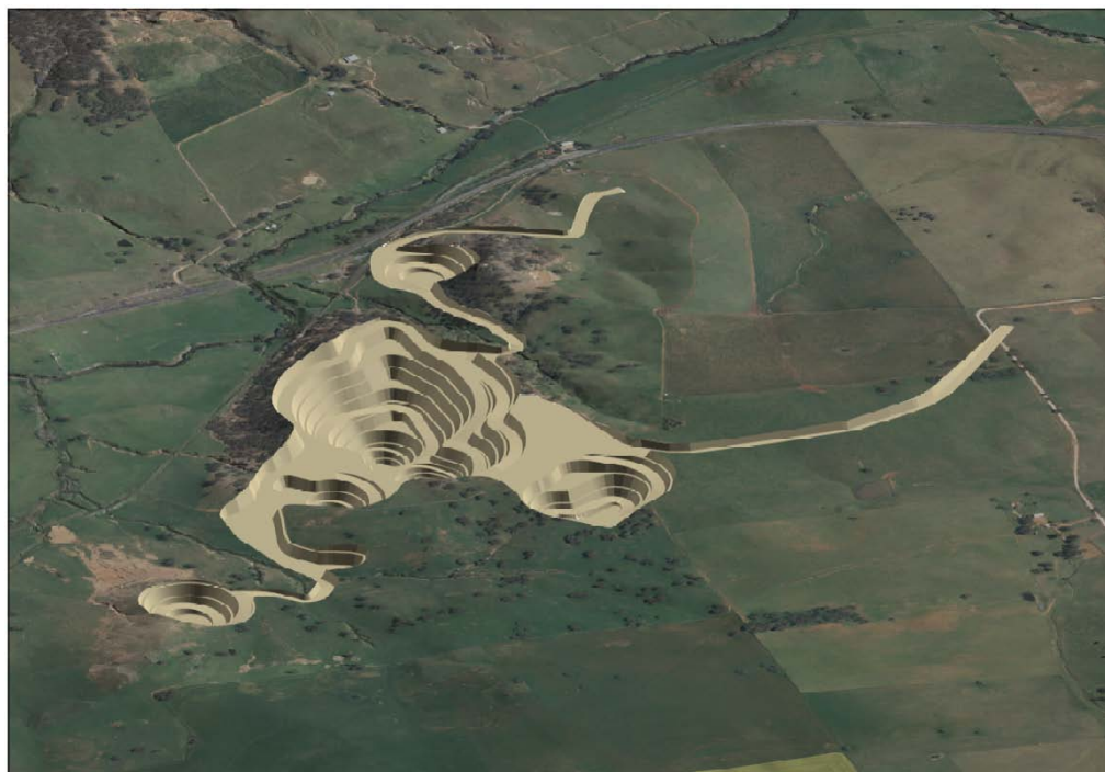
Figure 1. The potential 30Mt open pit containing average grades of 0.45% copper and 0.50g/t gold.
