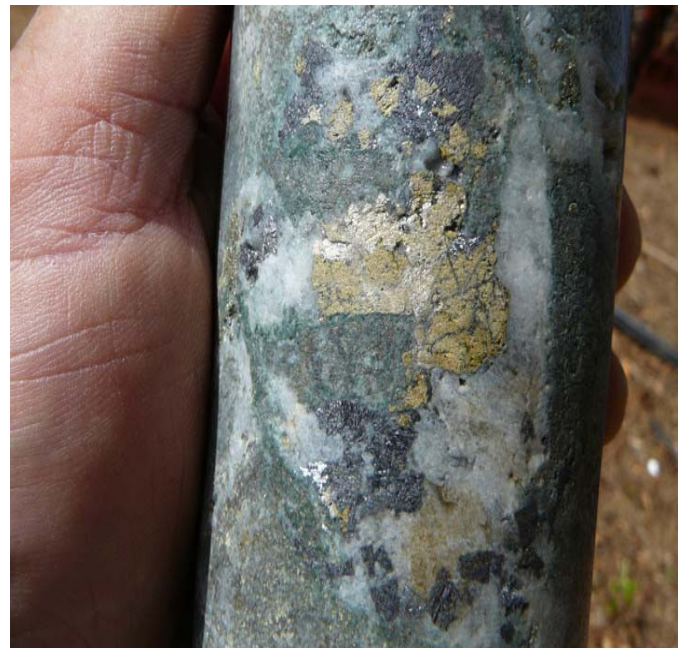
Photo 9 LHD-02 (97.50m) Close-up photo of quartz-base metal veining. The mineralisation seen here is principally sphalerite, with galena and trace chalcopyrite. Wall rock alteration is quartz-sericite pyrite, and the units are andesitic.
