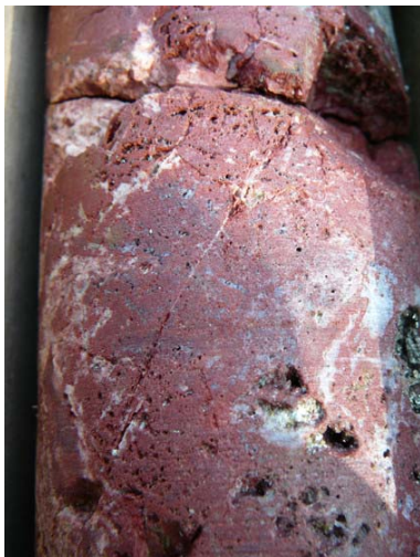
Photo 8 LHD-02 (68.10m) Quartz-hematite veining within altered andesitic sequences.
