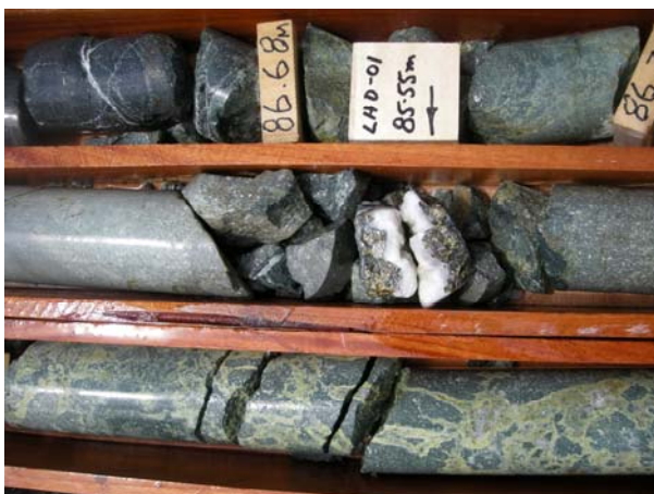
Photo 2 LHD-01 (85.55m) Quartz-base metal vein (quartz-pyrite-sphalerite-galena-chalcopyrite), approximately 4 cm wide, in a weakly altered andesitic sequence. The adjoining run (approximately 84.50m) shows pseudo-breccia textures in a propylitically-altered andesitic sequence.
