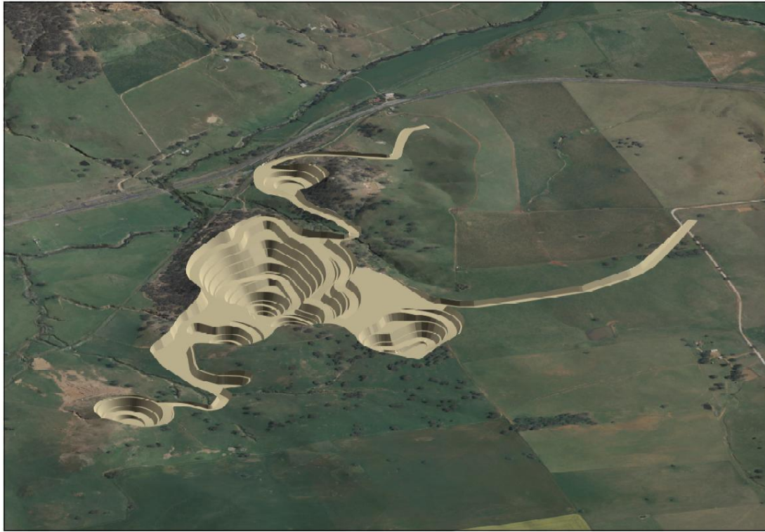
Figure 1. 3-D Schematic showing potential open pit containing 30Mt with average grades of 0.53% copper and 0.44g/t gold.
