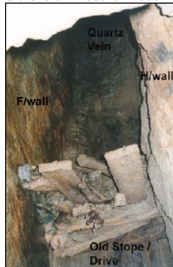
Figure 4 Sections through Challenger and old workings Section of H/w & F/w stopes
